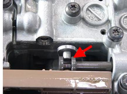
**Use hand tools - Do not use power tools for screw installation.**
