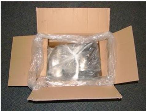
3. Place the mechatronic into a plastic bag to prevent oil leakage, then set into shipping box.
